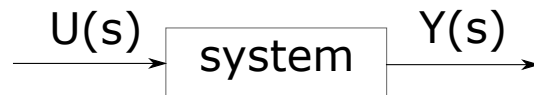
Figure 6: The input U(s) and output Y(s) to a system. The U(s) are for instance forces, the Y(s) are for instance positions.
